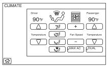
**Temperature**– Press the  $\triangle$  up and  $\nabla$  down arrows on the left side of the screen to increase/decrease the airflow temperature for the driver side of the vehicle. This control also adjusts the passenger side temperature when dual zone operation is disengaged.
